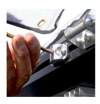
Finally insert the hook end of the rod into the hole on the awning.
