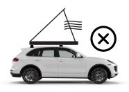
Never drive with the tent open as it can be dangerous and cause damage. Always place the opening towards the back of the car.
